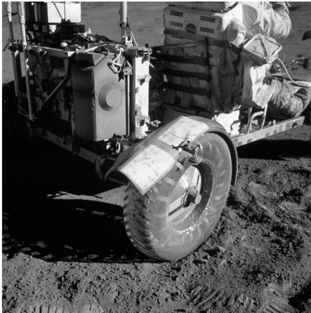
The Apollo 17 lunar rover fender, accidentally damaged by a rock hammer in Cernan's pocket, was repaired on the moon with a plastic-coated flight plan cover and duct tape. Photo Credit: NASA
