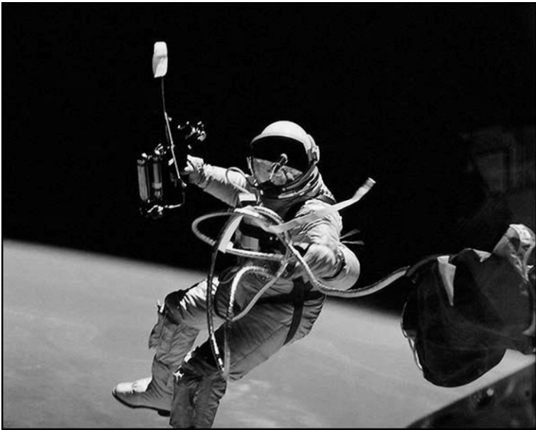
Astronaut Ed White uses the nitrogen-pressurized “zip gun” to propel himself during his Gemini 4 space walk on June 3, 1965. Photo Credit: NASA
