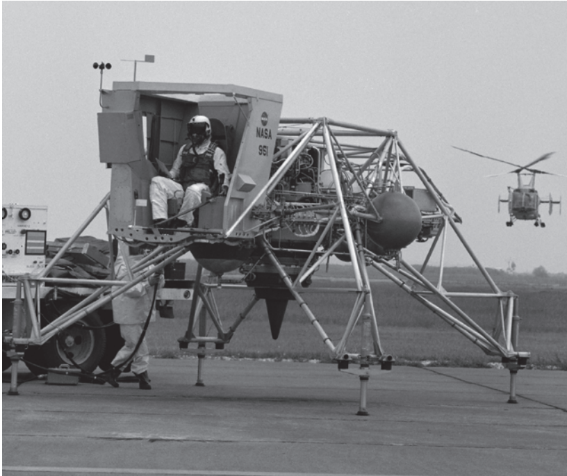
Apollo 11 Commander Neil Armstrong prepares for a training exercise in the Lunar Landing Research Vehicle (LLRV). Armstrong later bailed out of the machine seconds before it crashed. Photo Credit: NASA
